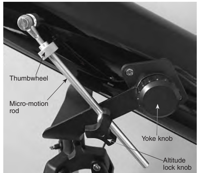
Figure 13. The micro-motion rod and thumbwheel allow fine altitude pointing control.
