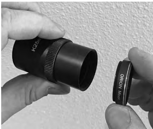
Figure 18. The Kellner eyepieces have barrels threaded to accept optional Orion 1.25" filters. A Moon filter is useful for cutting glare and revealing more detail on the lunar surface.
